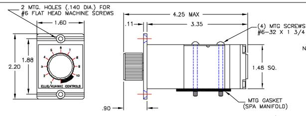
The PMT Series Pneumatic Timer is made to be used with most standard spool type (spring return—detented) valves of all leading brands of air logic. This timer has a logic output and is designed to operate the control pilot of the receiving valve. The timer is shipped as shown above with mounting screws and gasket. A subplate manifold (enables unit to be supplied with 10-32 or 1/8 NPT porting) is available but must be ordered separately.
