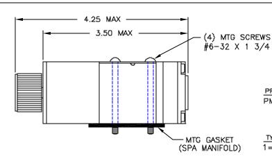
The PMT Series Pneumatic Timer is made to be used with most standard spool type (spring return—dented) valves of all leading brands of air logic. This timer has a logic output and is designed to operate the control pilot of the receiving valve. The timer is shipped as shown above with mounting screws and gasket. A subplate manifold (enables unit to be supplied with 10—32 or 1/8 NPT porting) is available but must be ordered separately.
