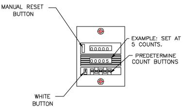
NOTE: TO SET PREDETERMINED COUNT HOLD DOWN WHITE BUTTON (DIRECTION INDICATED BY ARROW). THEN DEPRESS PREDETERMINE COUNT BUTTONS TO ACHIEVE REQUIRED AMOUNT. CORRESPONDING DIGIT WILL ADVANCE ONE COUNT EVERY TIME DEPRESSED. LOWEST COUNT MUST BE AT FAR RIGHT DIGIT.
